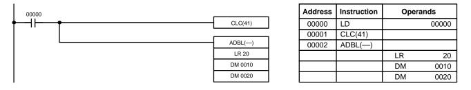
In the case below, 1,799,100,099 + (-282,751,929) = 1,516,348,100(6B3C167D + EF258C47 = 5A61A2C4). Neither OF nor UF are turned ON.
